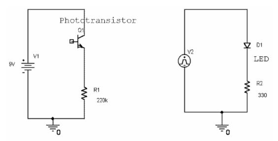
In the circuits shown above, Q1 a phototransistor (or possibly a photodiode, depending on what is in your kit) is an infrared detector and the LED (Light Emitting Diode) is an infrared transmitter. We will address the phototransistor circuit first.
