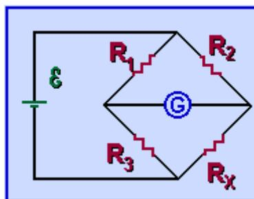
In this figure, taken from the Guelph tutorial, the capital E represents the voltage source (this letter is used a lot, but not as much as the capital letter V), and G represents some kind of measurement device. This circuit has been set up to determine the unknown resistor  $R_x$ , just as we did in Experiment 2.
