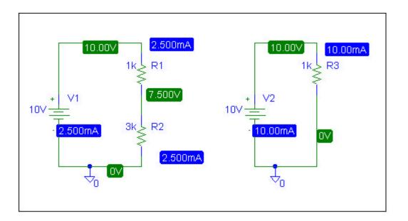
Plugging into the formulas on the previous page, we see that  $V_{Th} = 7.5$  volts, which agrees with the voltage at the point between R1 and R2 in the left diagram. The formula for  $R_{Th}$  gives 750 ohms. Using the PSpice results we obtain the same thing by taking the ratio of the open circuit voltage (7.5 volts) to the short circuit current (10mA from the right diagram). We can do the same kind of analysis with the bridge circuit.
