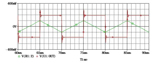
Note: In the VPULSE source model, V1 is the negative voltage for the pulse, V2 is the positive voltage, PER is the period, TD is a time delay from zero, TR is the time for the rising edge of the pulse, TR is the time for the falling edge of the pulse and PW is the width of the pulse.
