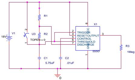
The circuit above has been simulated using PSpice. Using PROBE, the voltages at pins 2, 6, 7, and 3 have been displayed. Determine the values of resistors R1 and R2 from the information in this plot. Also, label which trace goes with which pin in each time period. Be sure that you label the traces in both the on and off parts of the pulse cylce.
