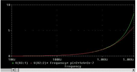
source. The AC sweep shown demonstrates that the circuit works like a differentiator for frequencies above 1kHz, since essentially both sides of equation 6-20 are plotted. The transient analysis again shows the differentiator is working at 1kHz, since the output voltage is 90° out of phase with the input.
