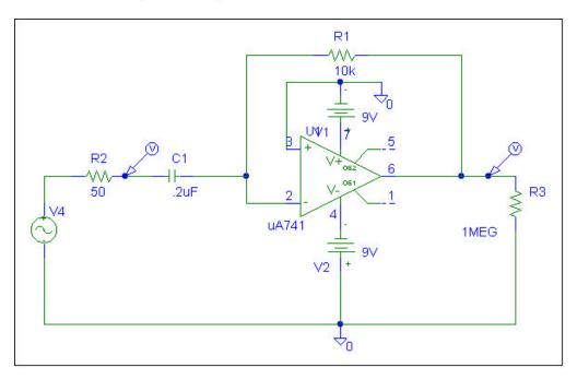
The only change to the circuit is the sinusoidal source rather than the pulse
