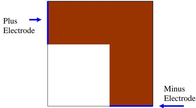
Assume that we have a thin conductor deposited onto the surface of a plastic board (as on a printed circuit board). The conductor is L-shaped, so any current passing through it must turn a corner. The square region in which the conductor is found is 10cm by 10cm. The conductor is 4cm wide and 1mm thick. To keep things simple, we will assume a conductivity of  $\sigma = 10$  as might be obtained using some kind of salty water solution.
