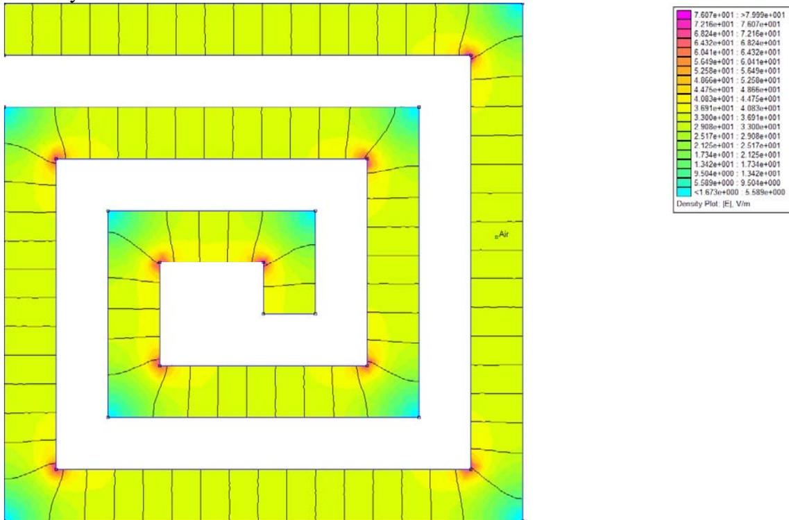
Label the regions in this plot where the electric field is the largest and where it is the smallest. Also note the regions in which the electric field intensity is reasonably uniform. Provide an explanation to accompany your labels.
