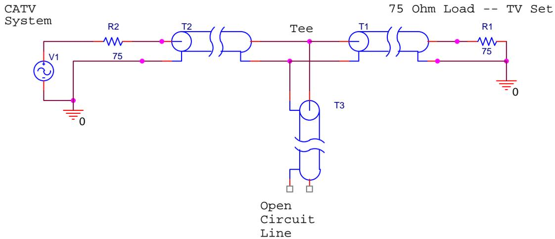
An open-circuited, 0.20 meter long transmission line with  $Z_o = 75\Omega$  and  $v_{ph} = 2.5 \times 10^8$  m/s connected to a CATV line with a Tee, as shown. Which of the following channels will be blocked by this line? (The frequencies are given in MHz.)
