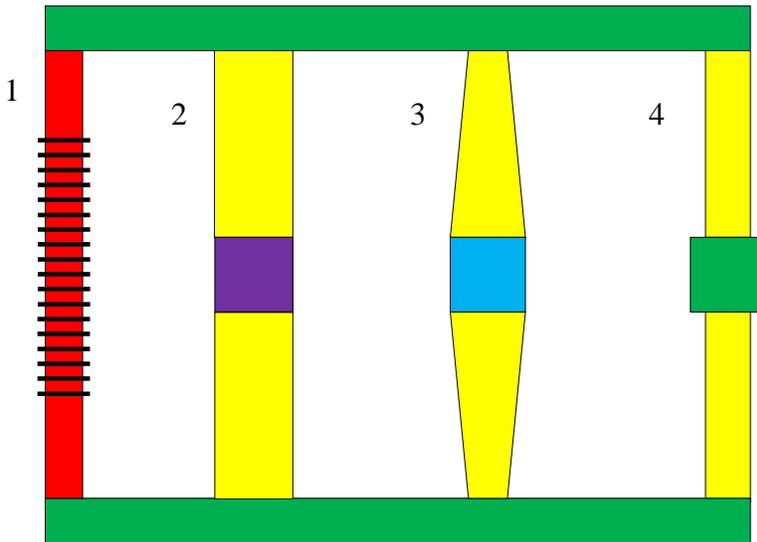
The magnetic circuit at the left consists of four legs. The leftmost leg is wrapped with  $N$  turns of wire carrying a current  $I$ . Each of the legs looks the same from each side. The square sections in the middle of the second, third, and fourth legs are identical cubes. The permeability of the cubes is  $\mu_{cube}$  and the permeability of all legs, including the horizontal legs at the top and
