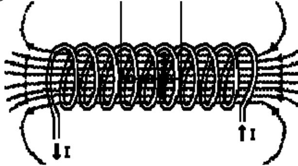
a. Making the assumption of no fringing effects (that is, treating the solenoid as a piece of an infinitely long cylindrical solenoid), determine the magnetic flux density  $\mathbf{B}$  everywhere in space. For now, leave your answer in terms of  $a$ ,  $d$ , and  $N$ . Do not plug in the numbers.
