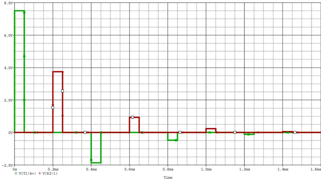
a. First, identify the input and output voltages in the diagram above. Then, determine the time it takes for the pulse to propagate from the input to the output of the transmission line. From this information, determine the relative permittivity  $\epsilon_r$  of the insulating material used in the cable.
