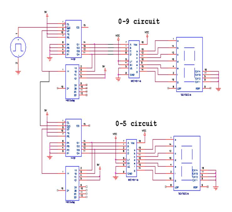
7.7 Instead of using the Function generator, use a 555 timer to trigger your clock circuit.
