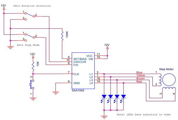
Pressing the button should advance the step motor. However, due to circuit 'bounce' the SAA1042 may try to advance the motor twice or more even if the motor is not capable of doing this quickly enough. If this is the case, try using a function generator to supply the clock pulses. Set the function generator to create a 1 Hz square wave with a 6 volt amplitude and a 3 volt DC offset.
