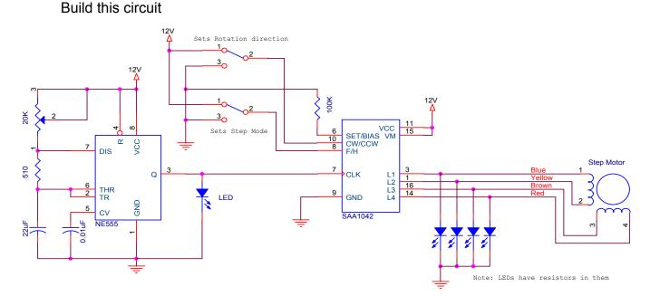
The TA will supply you with a 555 circuit. You will have to adapt it to be wired as shown above. If you used a function generator before, the 555 simply replaces it.
