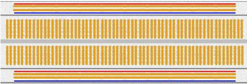
To use the bread board, the legs of components are placed in the holes. Each set of holes connected by a metal strip underneath forms a *node*. A node is a point in a circuit where two components are connected. Connections between different components are formed by putting their legs in a common node.
