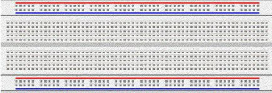
The bread board has strips of metal which run underneath the board and connect the holes on the top of the board. The metal strips are laid out as shown below. Note that the top and bottom rows of holes are connected horizontally while the remaining holes are connected vertically.
